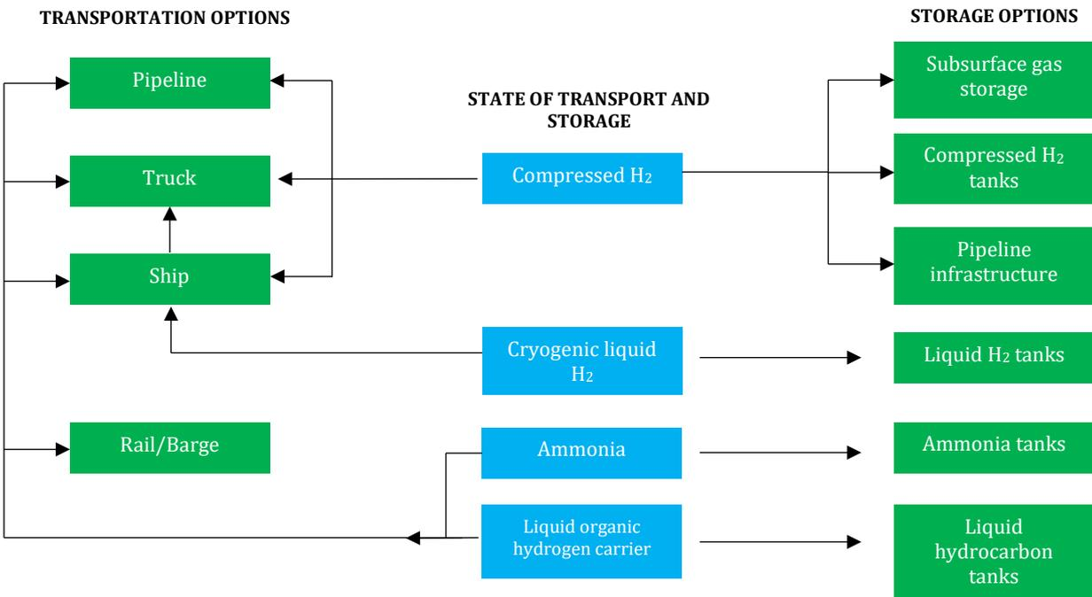
Figure 7 Main options for H<sub>2</sub> storage and transport<sup>28</sup>
