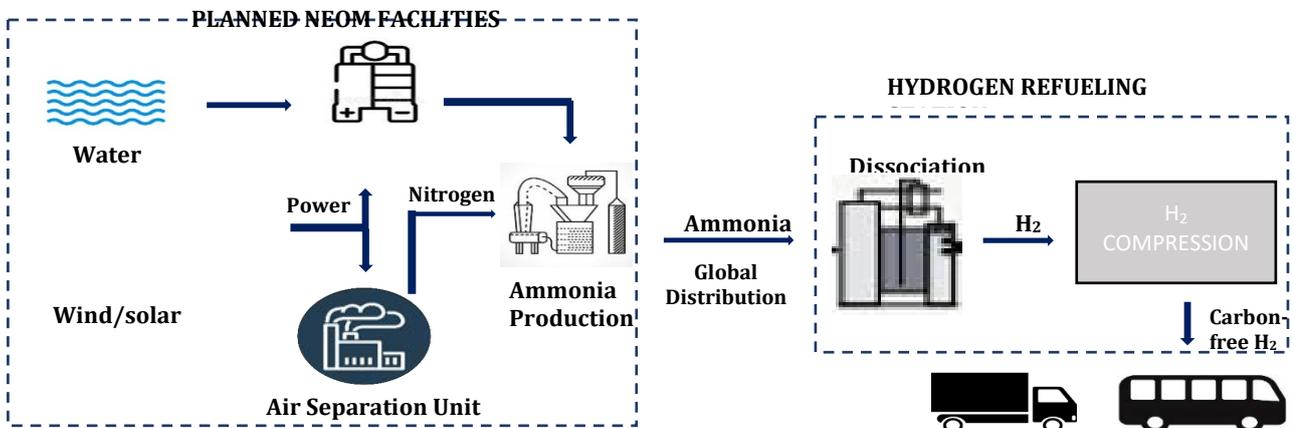
Figure 15 Neom planned H<sub>2</sub> production, transport and application
