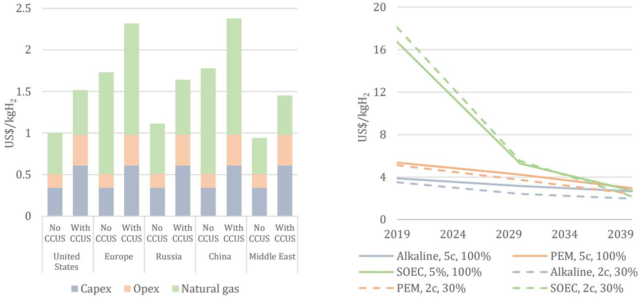
Figure 6 Hydrogen production costs using natural gas<sup>26</sup> versus hydrogen production costs using electrolysis<sup>27</sup>
